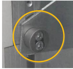
Fig. 56 Bushing LB 18-2-SL13-2xM5x16.
