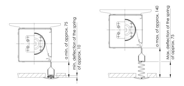
**Note**: Keep the minimum and the maximum deflection of the spring. The dimension between the casing and the ceiling is approximate.
