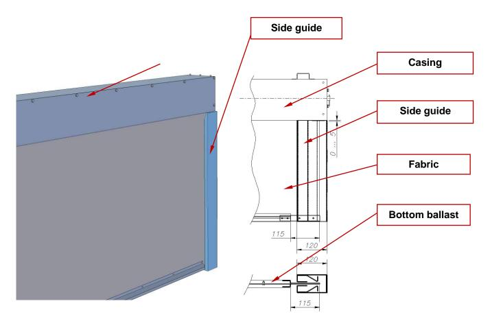
Fig. 22. Method of installing side guides.
