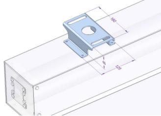
Flat bracket – TYPE C (fixed only directly to the ceiling)
