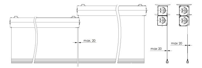
Fig. 14. Typical sizes of gaps in the traverse direction with the curtain modules arranged vertically and without the fabric overlapping
