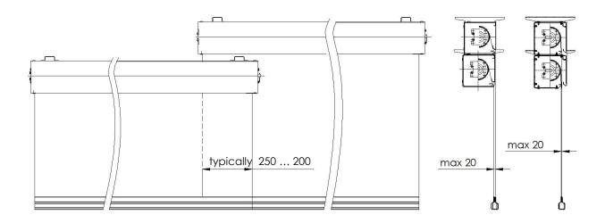
Fig. 13. Typical sizes of gaps in the traverse direction with the curtain modules arranged vertically and with the fabric overlapping.
