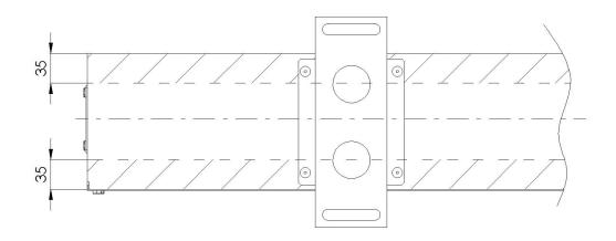
Fig. 10. Place on the casing intended for joining the curtain modules
