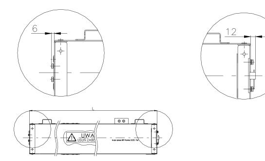
Fig. 2. Length of the elements protruding from the casing of the *mcr PROSMOKE CE/CE1* curtain.
