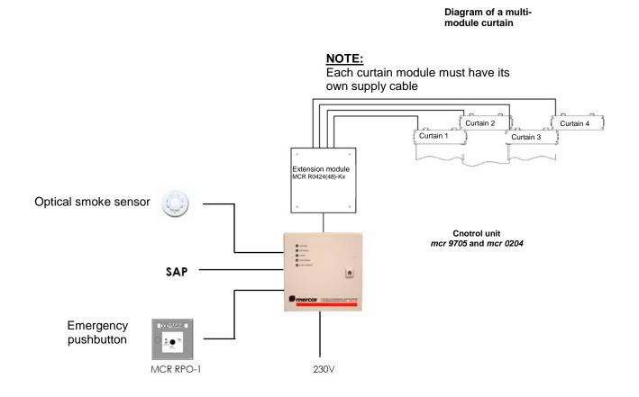
Fig. 11. Schematic diagram of the connections of a curtain with common bottom ballast
