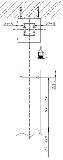
Fig. 9. Installation of a curtain without a bracket
