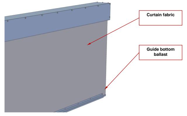
Fig. 21. Curtain ready to have side guides fitted.
